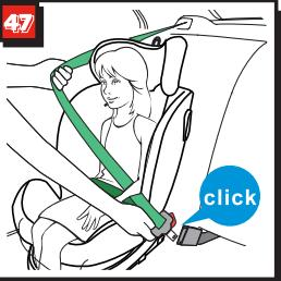
Have your child sit down in the child seat. Adjust headrest in proper height (see section 4.3). Pull out the vehicle seat belt and guide it in front of your child to the vehicle seat buckle. Engage the buckle tongue in the vehicle seat buckle. (fig.47)
