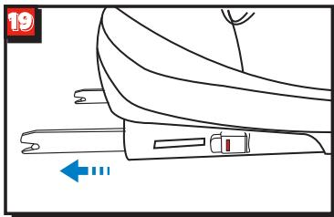
On both sides of the baby car seat squeeze ISOFIX button and pull out ISOFIX in longest position.
