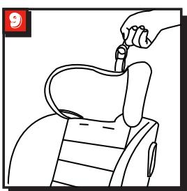
First loosen harness. Pull up the headrest height adjuster at the same time move headrest to shoulder height in accordance with the size of the child. (fig.9)
