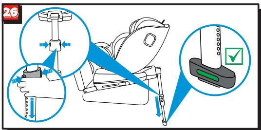
Pull the support leg away from the bottom of the baby car seat until fully extended. Push both adjustment buttons and pull out the support leg until it rests firmly on the floor of the vehicle. Make sure the indicator on the support leg must turn green, the bottom of the baby car seat does not lift up from the surface of the vehicle seat and two adjustment buttons must be fixed.
