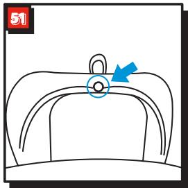
Loosen the press studs at the back of the headrest and remove the cover of headrest.
