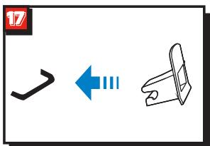
If your vehicle is not equipped with ISOFIX insert guides as standard, clip the two insert guides which are included with the baby car seat, with the cut-out facing upwards onto the two ISOFIX attachment points of your vehicle.
