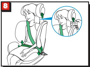
When fixed by 3-point vehicle belt, the headrest must be adjusted so that there is a space two fingers wide between the headrest and your child's shoulders. Make sure the diagonal seat belt section is on child's shoulder but not on neck. (fig.8).
