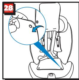
Loosen the press studs on the backrest and fold the upper half of the cover upwards and the lower half downwards. (fig.28)
