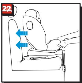
Slide the two ISOFIX firmly into the insert guides until ISOFIX engage with a clicking noise on both sides. ISOFIX indicator must turn green on both sides. (fig.20,21)
