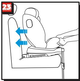
Push the baby car seat towards the backrest applying firm. (fig.23)
