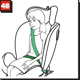
Place the diagonal seat belt section and lap belt section on the side of the vehicle seat belt buckle in the lower belt guide. (fig.48)
