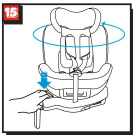
Pull rotation button at the same time rotate baby car seat to intend direction. (fig.14,15)
