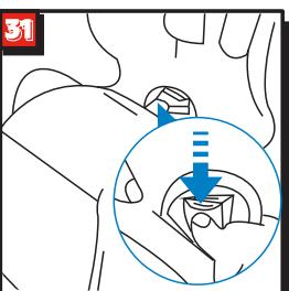
Pull the harness buckle out of the cover. (fig.31)
