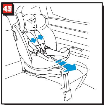
Have your child sit down in the child seat. Adjust headrest in proper height (see section 4.3), adjust harness and lock buckle, and tighten harness (see section 4.1, 4.2). (fig.43)
