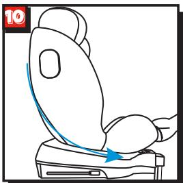
Baby car seat has five recline positions. For rearward facing, only use most reclined position. For forward facing, can use all five positions. Except most upright position, other positions may not fit in all approved vehicles. Pull recline lever at the same time incline baby car seat to intend position. (fig.10)
