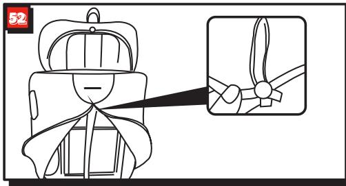
Loosen the press studs and unzip at the back of seat cover. Pull forward and remove seat cover.
