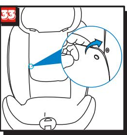
Fasten the top and bottom of the cover back. (fig.33)
