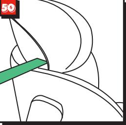
Guide the diagonal seat belt section into the Belt holder and it is not twisted. (fig.50)
