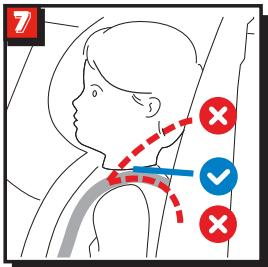
When fixed by 5-point harness, the headrest must be adjusted so that the shoulder belts are at the same level as your child's shoulders. (fig.7)
