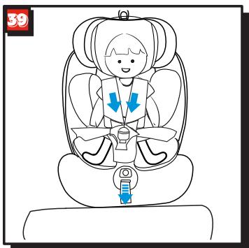
Have your child sit down in the child seat. Adjust headrest in proper height (see section 4.3), adjust harness and lock buckle, and tighten harness (see section 4.1, 4.2). (fig.39)
