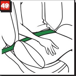
Place the lap belt section on the other side of the child seat in the lower belt guide. (fig.49)
