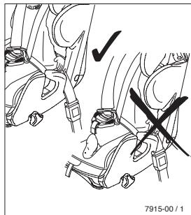
Regardless of whether it is being used for age group I or II+III, ensure that the belt position is correct at the load-bearing points. The buckle must always be below the belt guide.
